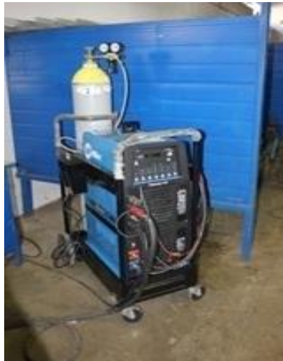
Figure 5-12: poste de soudage TIG (CRTI)
