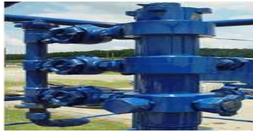
Figure III.5: Tête de cimentation [1].
