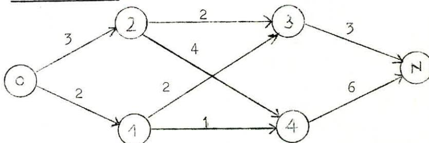
$$\begin{array}{llll} t_1 \geq 2 & t_3 - t_1 \geq 2 & t_3 - t_2 \geq 2 & t_n - t_3 \geq 3 \\ t_2 \geq 3 & t_4 - t_1 \geq 1 & t_4 - t_2 \geq 4 & t_n - t_4 \geq 6 \end{array}$$
