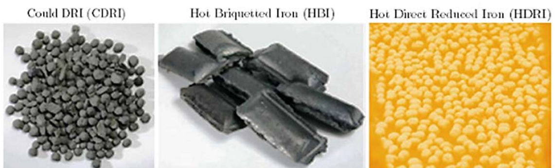
Figure 29 : Différents types de DRI (directement de MIDREX) Source: P. Cavaliere, Clean Ironmaking and steelmaking processes
