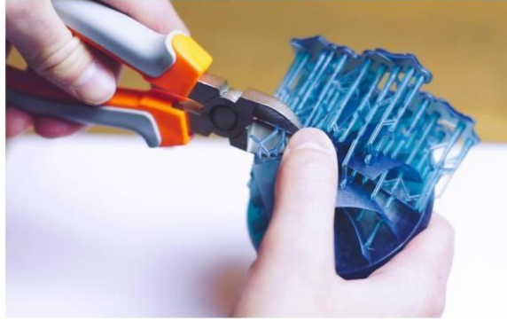
Figure 2.15: 3D printed object with support structures. [55]
