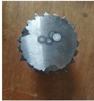
Figure 3-6: traces of spark spectrometry
