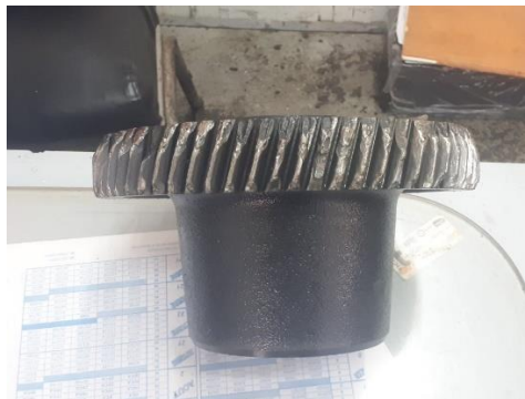
Figure 1-36: Tooth breakage defect on the crown gear
