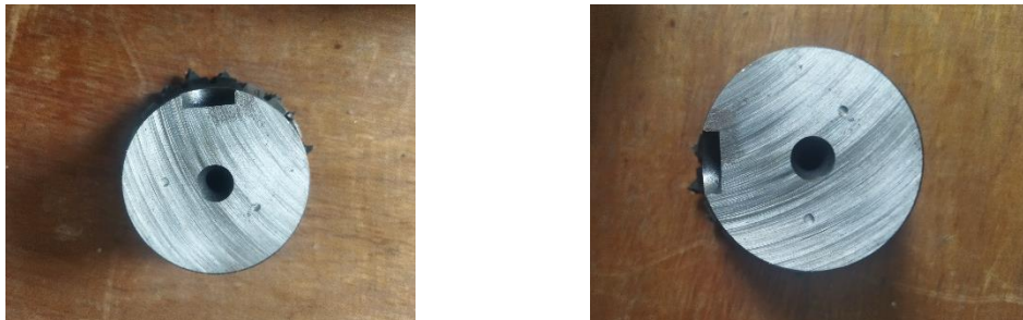
Figure 3-9: Brinell hardness test traces
