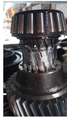
Figure 1-34: Tooth breakage defect (early phase) Figure 1-35: Tooth breakage defect (advanced phase)
