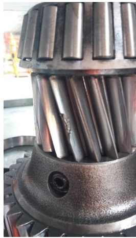
Figure 1-34: Tooth breakage defect (early phase) Figure 1-35: Tooth breakage defect (advanced phase)
