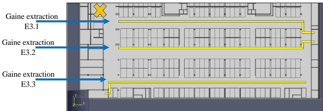
Figure 4.22 Compartiment 3 gaines d'extraction 2D
