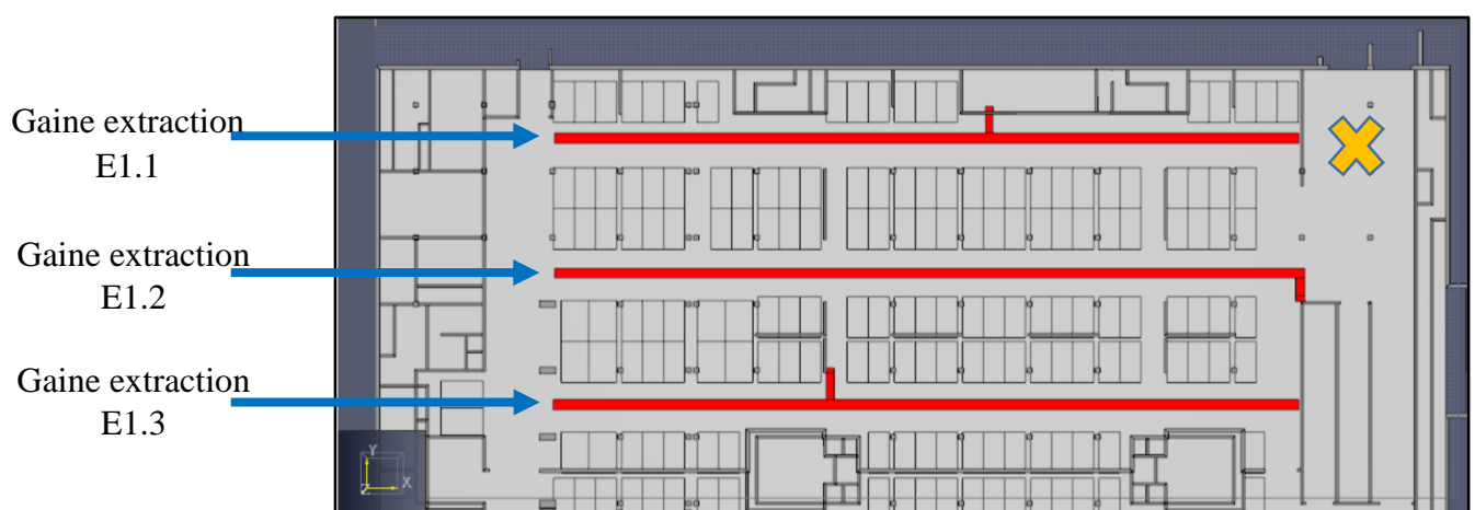
Figure 4.18 Compartiment 1 gaines d'extraction 2D
