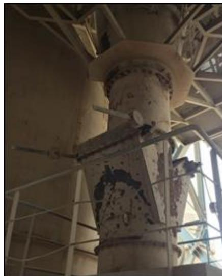
Figure 3-12 : Clapet papillon [26]
