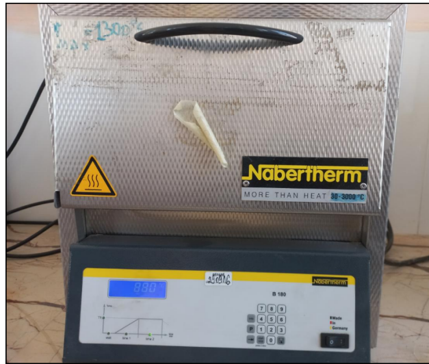
Figure 4.3: Nabertherm oven used for austenitizing and tempering.
