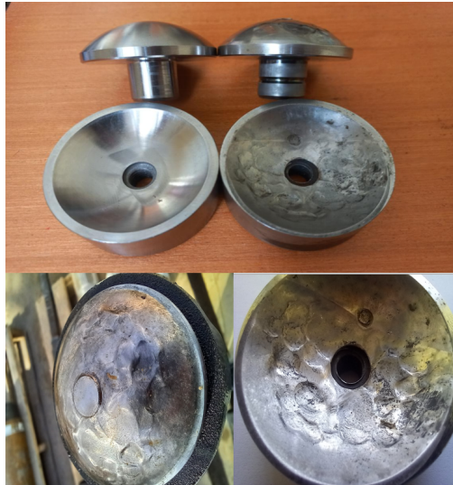
Figure 1.10: New thrust pin and insert compared to damaged ones.
