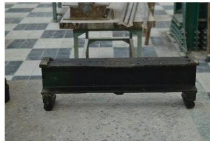
Figure d. Load distributor
