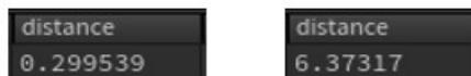
Figure 2.23: Model before (left) and after (right) scale calibration (Length of the bottom rectangular base).
