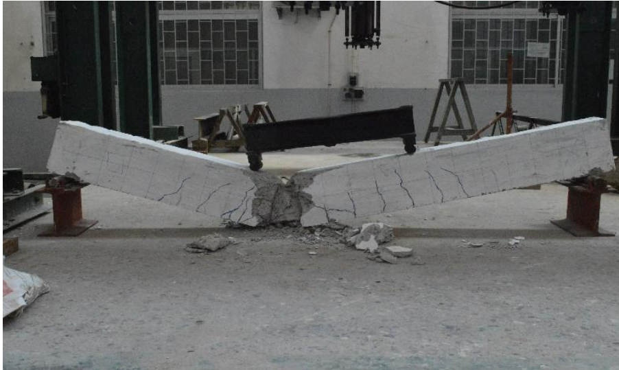
Figure 3.26: Beam after reaching failure.
