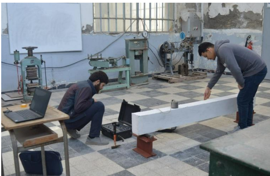
Figure 3.11: Ambient vibration test during recording.
