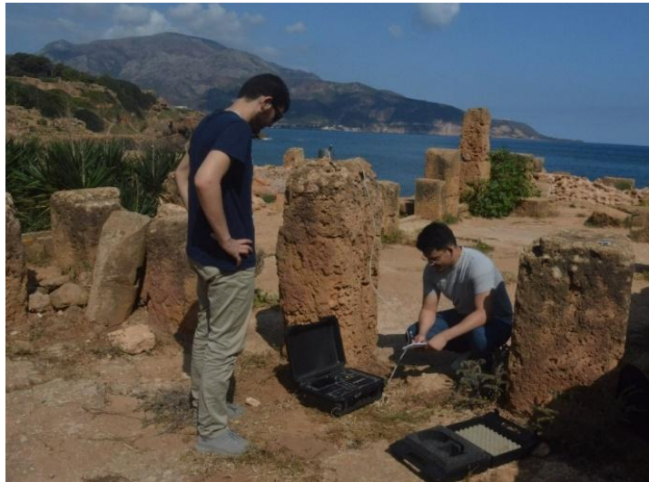
Figure 4.9: Ambient vibration test during recording on Tipaza historical site.
