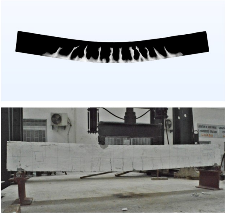
Figure 3.44: Comparison between simulated and experimental cracking pattern.
