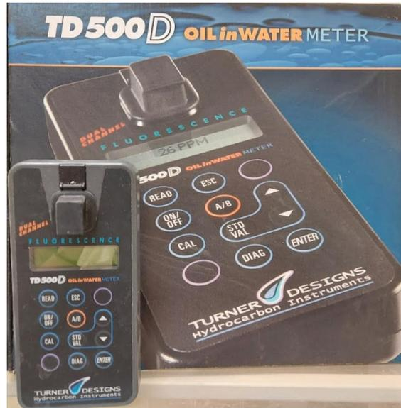
FIG. 4.1 : Appareil de mesure TD-500D oil in water meter
