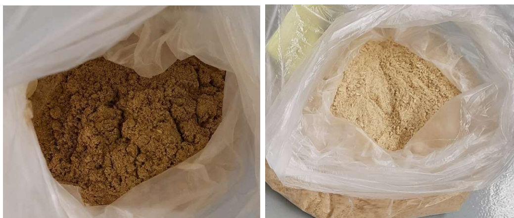
Figure 24: the result of the preparation for biosorbents based on Fennel seeds on the left and Sweet Thapsia on the right
