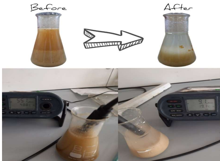
Figure 25: The difference on turbidity and electric conductivity before and after
