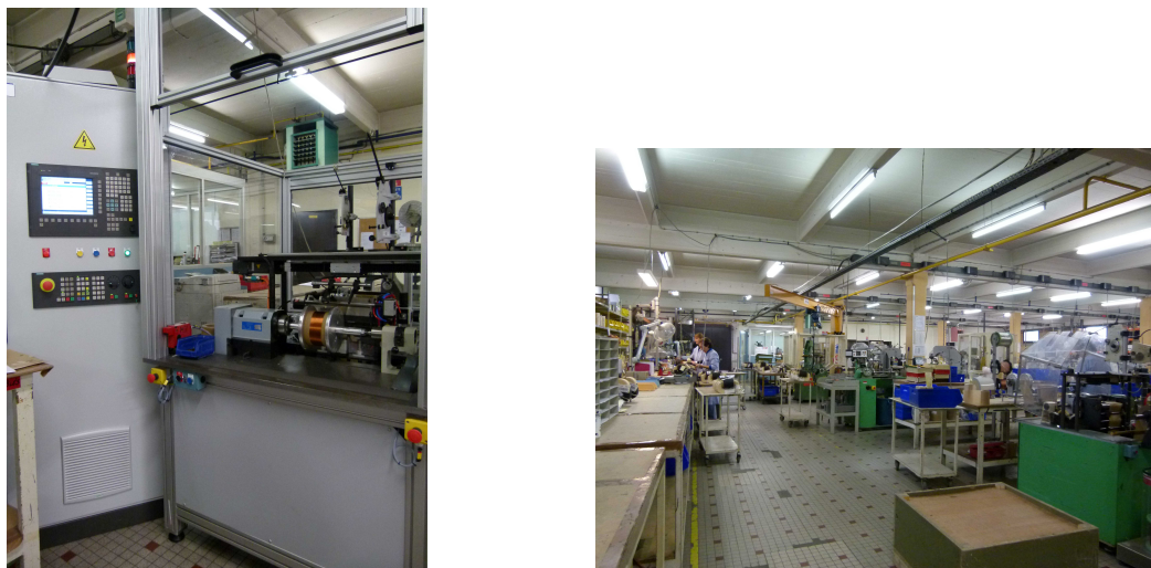
FIGURE 3.2 – Machines de bobinage
