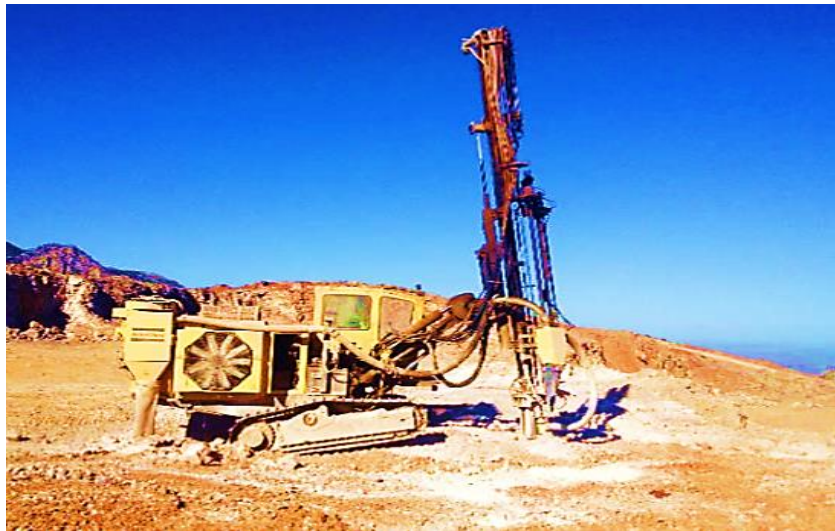
Figure IV. 4. Chariot de foration (Photo carrière Cosider).
