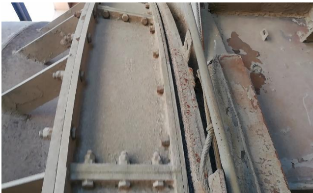
Figure 6. 6 Joint amont du four rotatif
