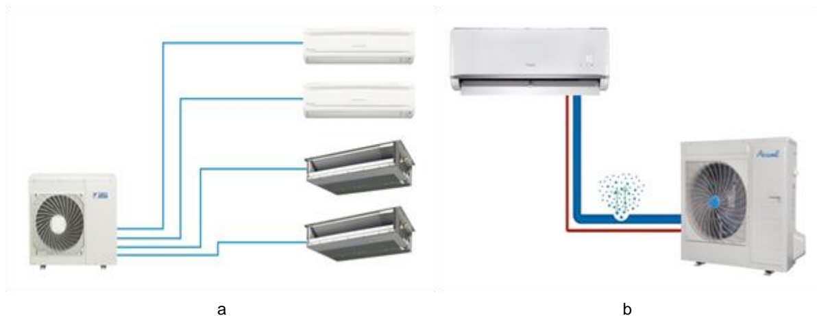
Figure 3.1 Climatiseur : (a) multi-split, (b) mono-split
