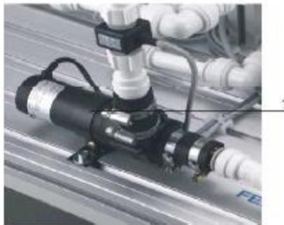
**Figure I.5 Pompe centrifuge**
