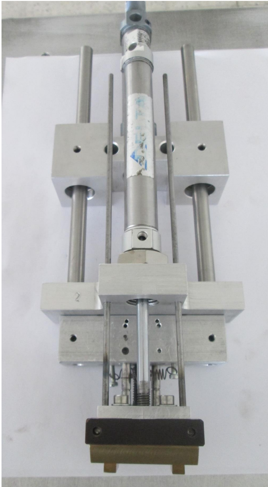
Figure 2.40: Y-axis motion assembly with pick-up and thermal fixation assemblies.
