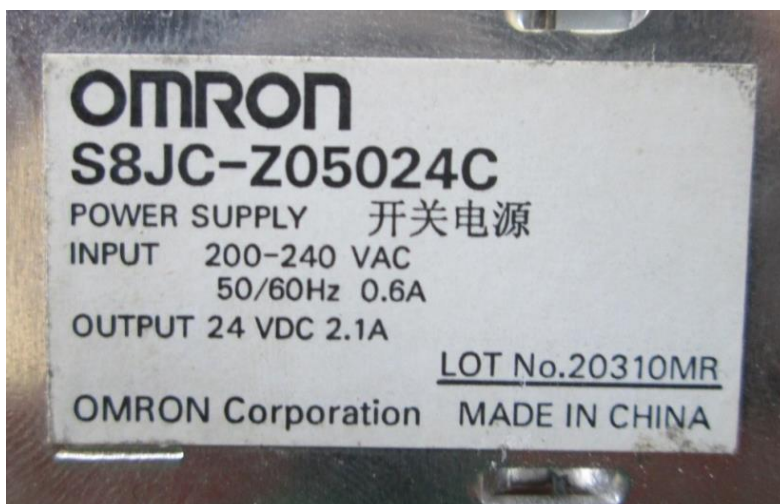
Figure 1.35: Omron S8JC-Z05024C Power supply nameplate.
