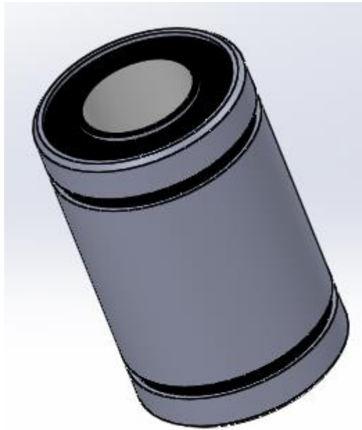
Figure 2.21: Im10uu linear roller bearing Solidworks model.
