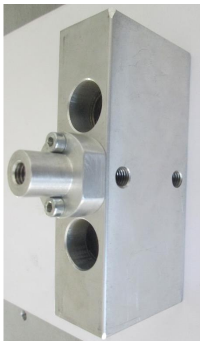
Figure 2.25: Moving piece with rod fixation assembly.
