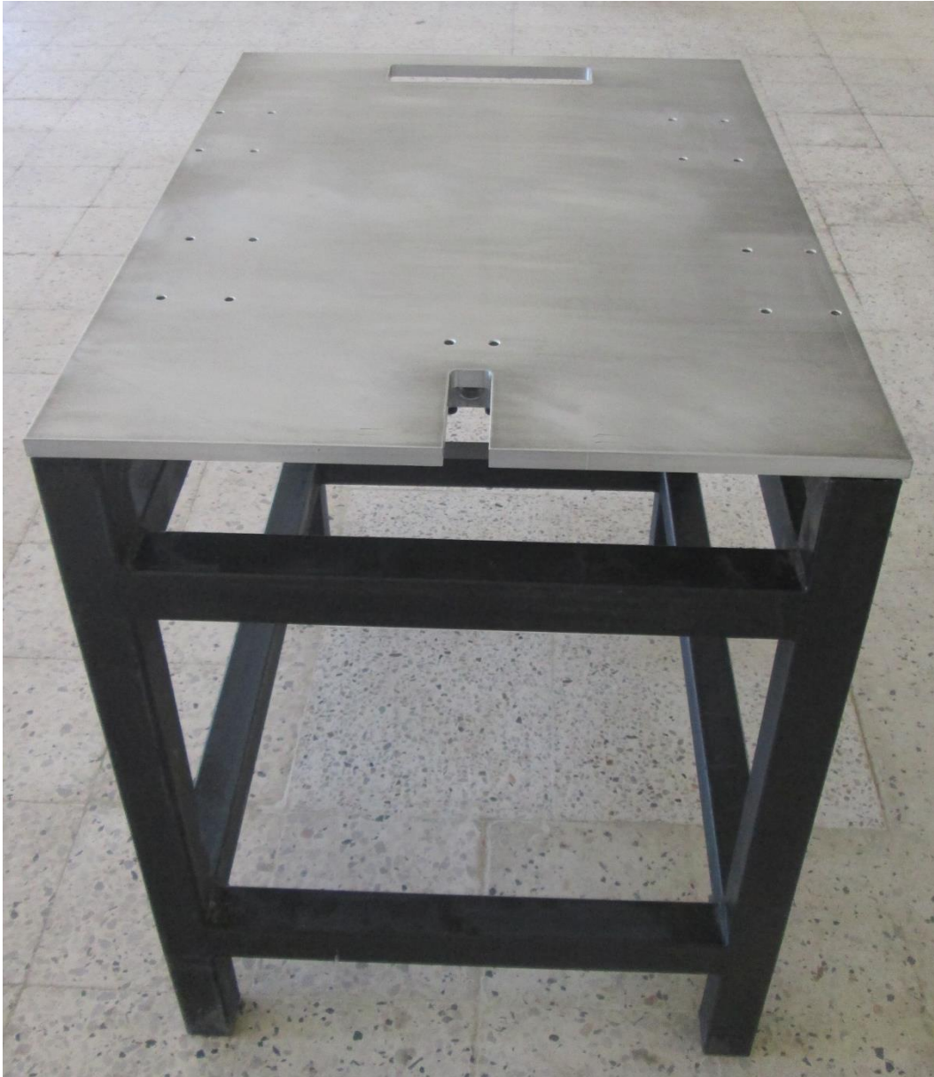
Figure 2.6: Worktable and Support base assembly.
