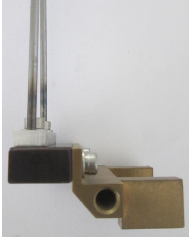
Figure 2.38: Thermal fixation system assembly.
