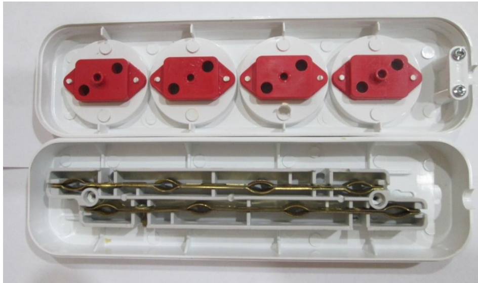
Figure 1.13: internal components of a power strip.
