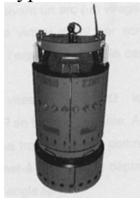
Figure I.16. Robot mobile B21r à traction synchrone.
