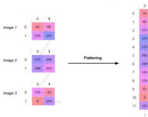
FIGURE 2.13: Illustration de l'opération flattening.
