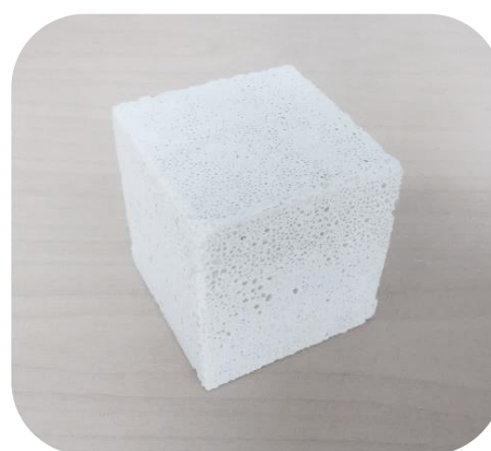
Figure 3.18: Epreuve cubique 70×70×70 mm
