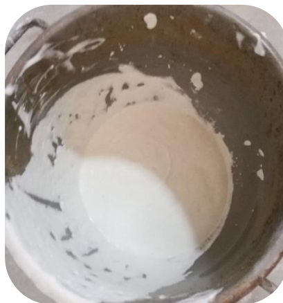
Figure 3.13: Coulis de ciment
