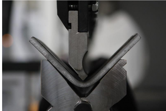
Figure 1-2 Cold-forming tools: brake press dies [16]
