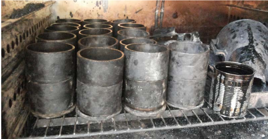
Figure 3.22: Etuvage du bitume
