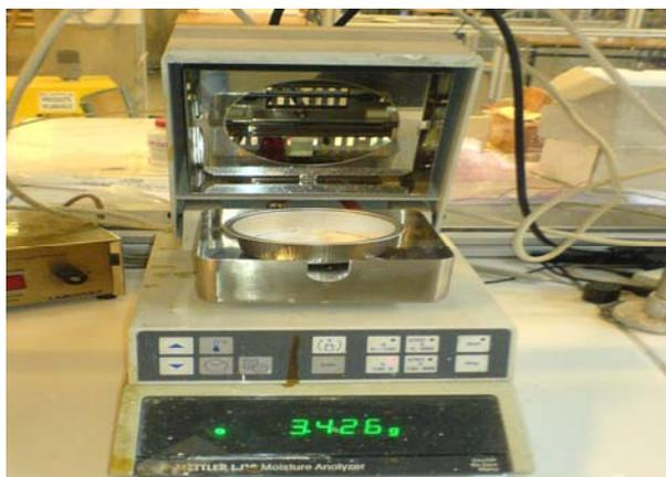
**Figure V.2 :** Photo de thermobalance Mettler U16 Moisture Analyzer
