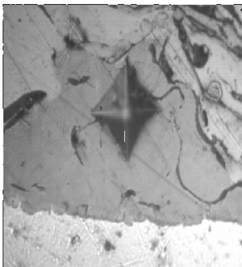
Figure VI.6: Empreinte du composite Thermanit/NiAl/AG3.
