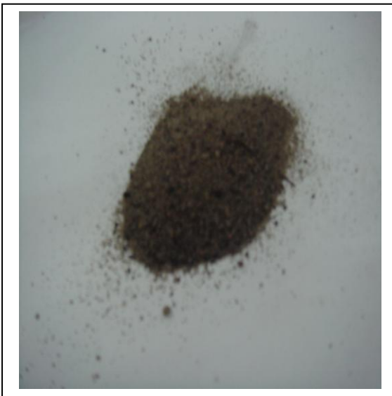
Figure II-2 : La pate bore-silicium.
