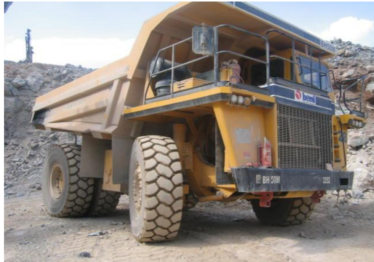
Fig.II.3: Dumper de carrière BEML BH 50M.
