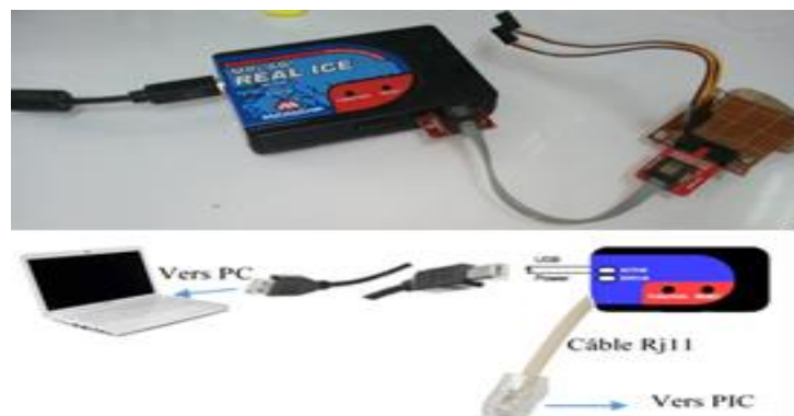
Figure 6.29. MPLAB Real ICE, Câblage du kit ICD
