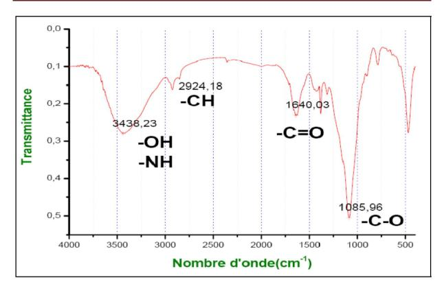
Figure V.3 Spectre infrarouge de la biomasse Pleurotus Mutilus
