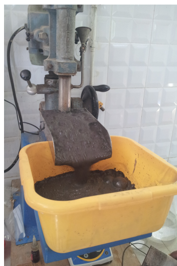
FIGURE 3.2 – Cellule de flottation (DENVER)
