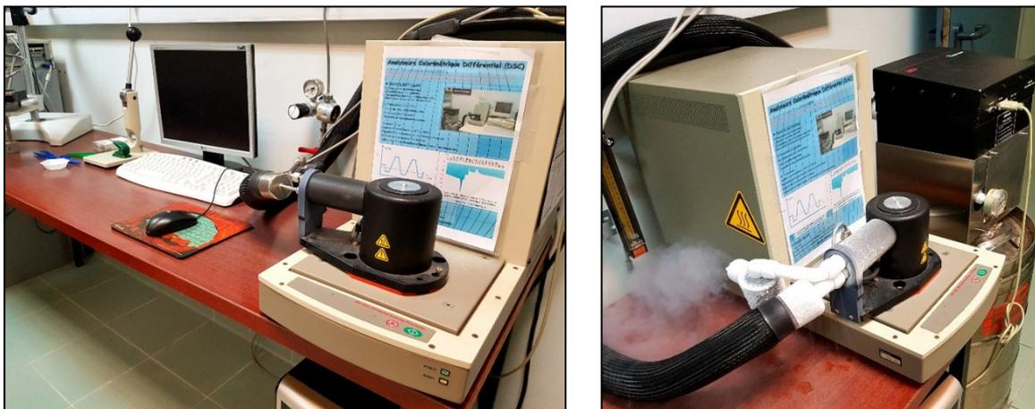
Figure II.5. Measurement and control equipment of DSC 2010 (LAPLACE)
