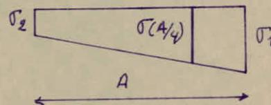
$$\begin{aligned} \sigma'_1 &= \frac{N}{S} + \frac{M_y}{I_y} v_{y_2} = 1,71 \text{ bar} \\ \sigma'_2 &= \frac{N}{S} - \frac{M_y}{I_y} v_{y_1} = 0,70 \text{ bar} \end{aligned} \quad \left. \right\}$$
