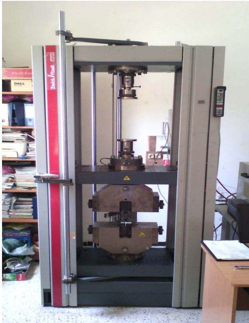
Figure II.12: Machine de traction Zwick/Roell.
