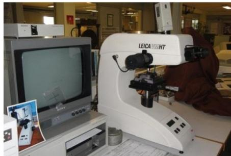
Figure 4-17: Image microdurometre Vickers Leica VMHT.
