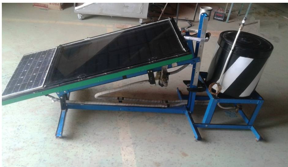
Fig. 3. The realized prototype of the developed solar water heater.
