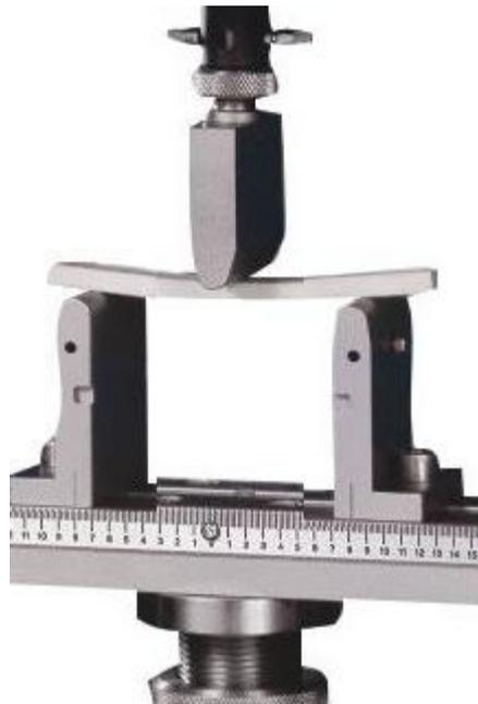
*Dispositif Eprouvette ASTM 2017 /ASTM301*
