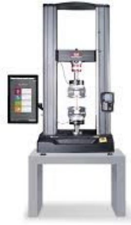
**Figure 1.9 . Machine universelle de traction multi colonnes**
