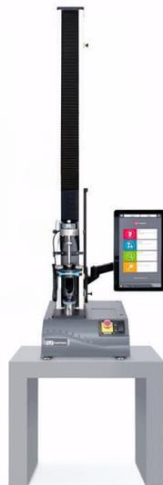
Figure 1.8 . Machine universelle de traction mono colonne
