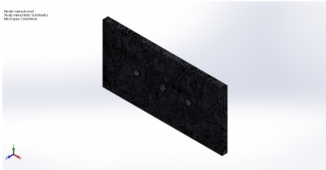
FIGURE V.12: Discretization of the Aluminium Plate
