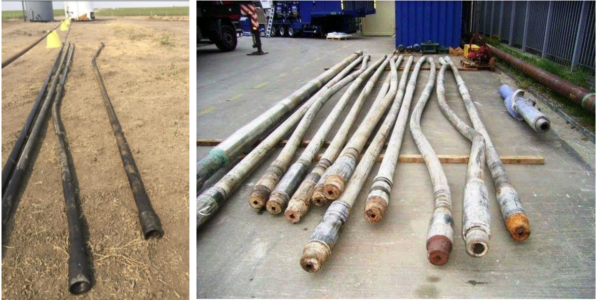
Figure 2-3 The picture of drill pipe buckling
