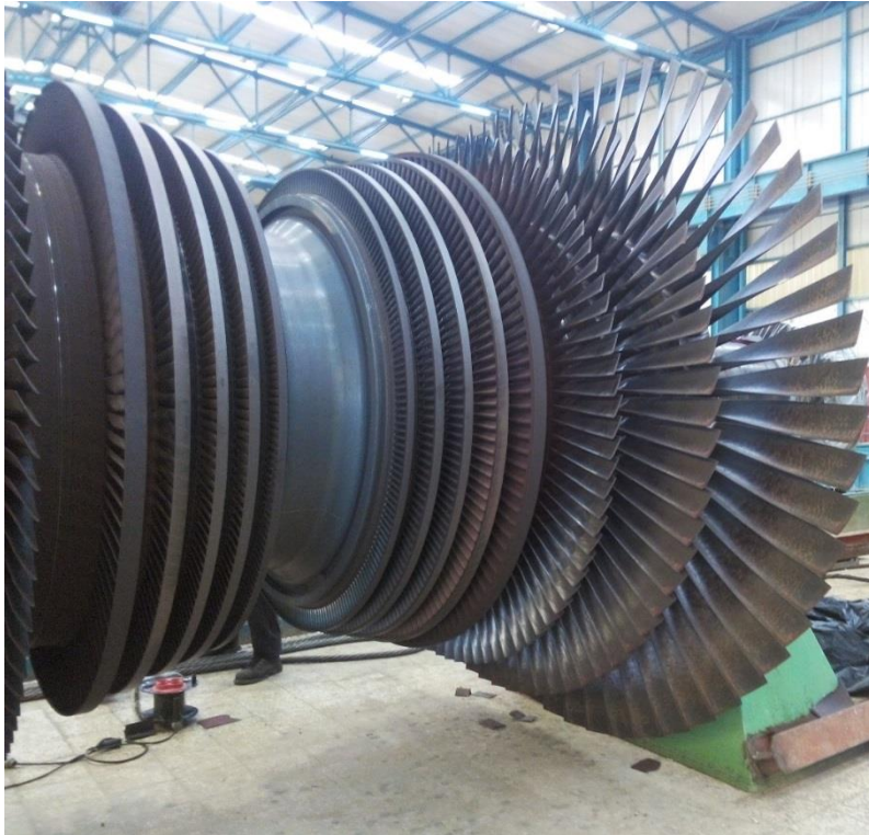
Figure IV.5: Corps BP de la turbine
