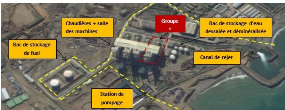
Figure I.4: Disposition de la centrale (I.5)
