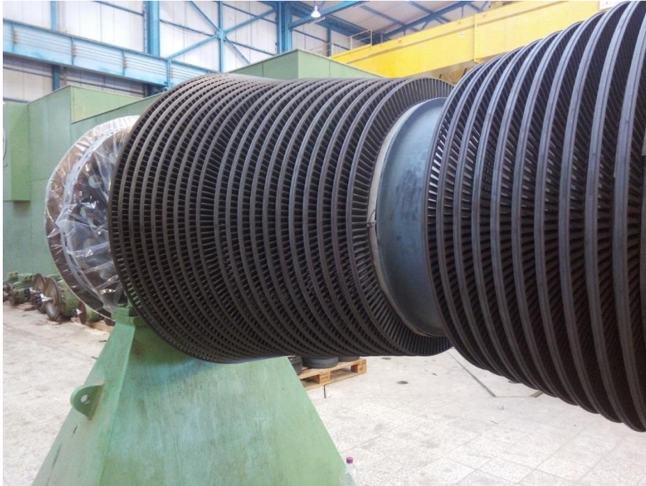
Figure IV.3: Corps MP de la turbine
