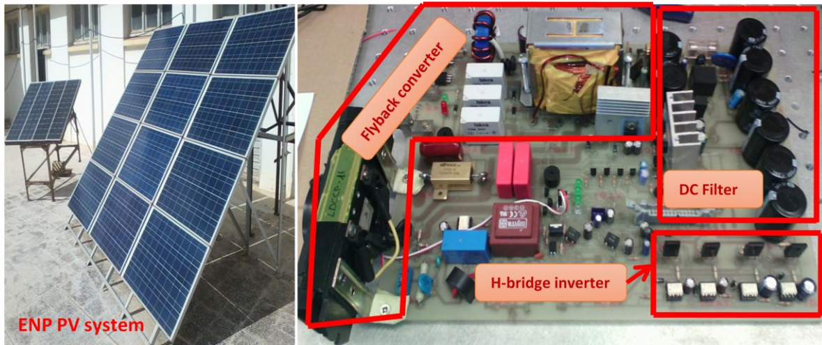
Fig 4.17 Final experimental PV inverter card.
