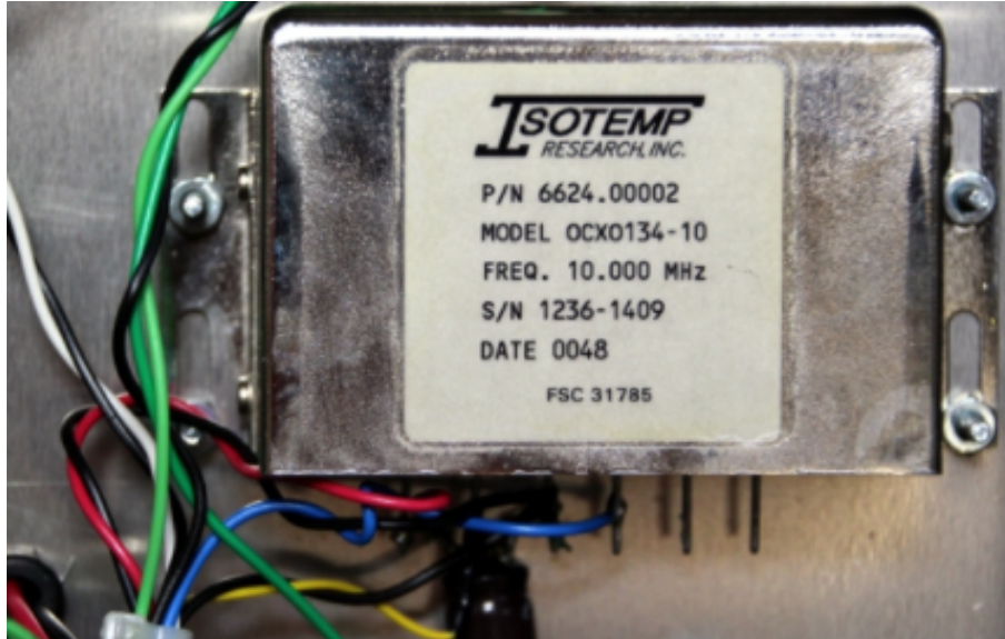
Figure 1.3: oven controlled quartz oscillator
