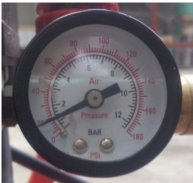
(a) pressure on the compressor barometer.
