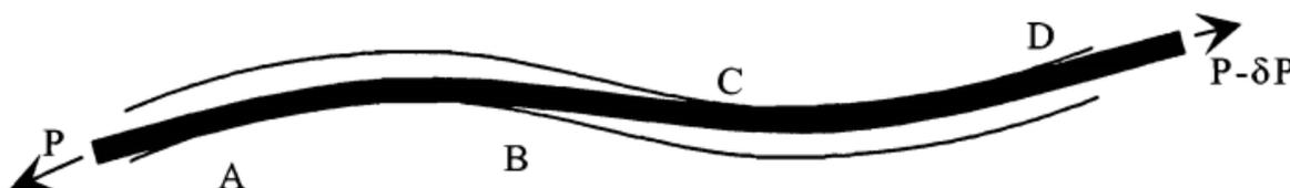
Fig VI-25 Position relative du c  ble et de la gaine
