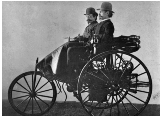
Figure 1.3 Patented in 1886 by Karl Benz, the Motorwagen was the first vehicle designed to be powered by an internal combustion engine. Source: History center website (37)
