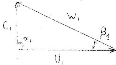
$$\begin{aligned} \implies W_1 &= \sqrt{C_1^2 + U_1^2} \\ &= \sqrt{3,8^2 + 11,5^2} \implies W_1 = 12,11 \text{ m/s} \end{aligned}$$
