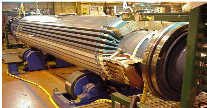
Fig.I.13. Rotor de 450 H Generator (GE) [9]
