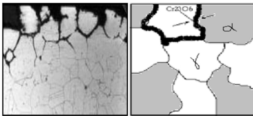
Figure I.9: corrosion intergranulaire.
