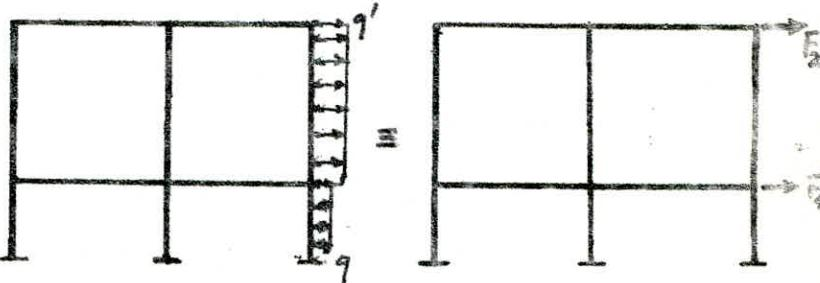
$$\text{efforts tranchants: } T_2 = F_2 = 1,52 \text{ tf.} \quad T_1 = F_1 + F_2 = 3,30 \text{ tf.}$$
