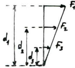
$$d_1 = 495 \text{ mm}, \quad d_2 = 315 \text{ mm}, \quad d_3 = 135 \text{ mm}.$$
