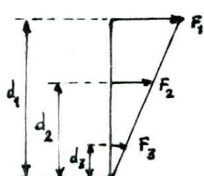
$$d_1 = 260 \text{ mm.} \quad d_2 = 160 \text{ mm.} \quad d_3 = 60 \text{ mm.} \quad F_i = \frac{M \cdot d_i}{\sum d_i^2}$$
