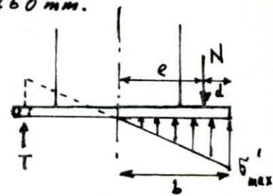
$$\tilde{\sigma}_{\max}' \times \frac{15 \times 46}{2} = N. \Rightarrow \tilde{\sigma}_{\max}' = \frac{2 \times 47000}{15 \times 46} = 136 \text{ daN/cm}^2.$$
