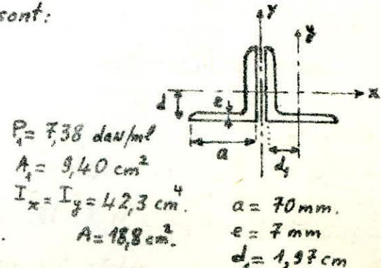
(3) Entrait:  $N' = 90 \text{ t}_f$  (traction).  $l_o = 1,50 \text{ m}$ .  $l_{q_x} = 4 l_o = 6,00 \text{ m}$ .
