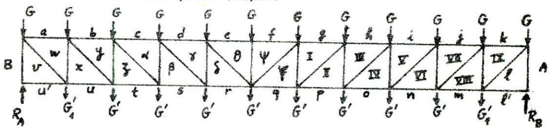
$$G = 2,5 \text{ tf}, \quad G' = 0,73 \text{ tf}, \quad G_i = 1 \text{ tf}, \quad R_A = R_B = 19 \text{ tf}.$$
