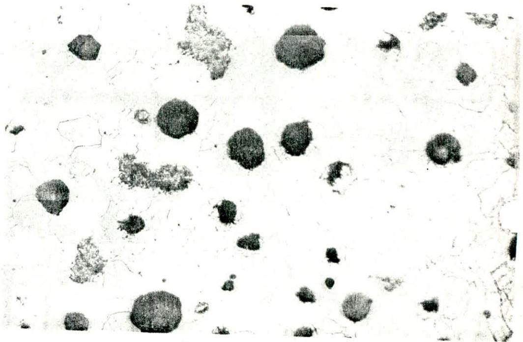
Fig 5.4: STRUCTURE FERRITIQUE/
